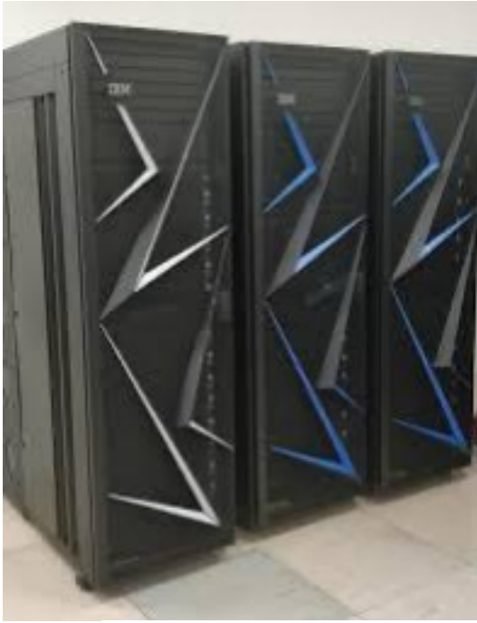
Fig. 10. MARCONI 100 is the new accelerated cluster based on IBM Power9 architecture and Volta NVIDIA GPUs, acquired by Cineca within PPI4HPC European initiative.
