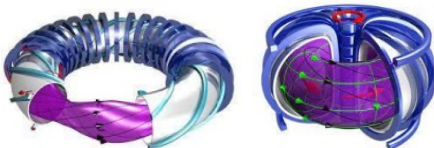
Fig. 3. The two main concepts of magnetic confinement fusion: a stellarator (left) and a tokamak (right)
